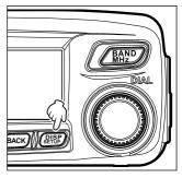
2 Rotate the DIAL to select [4 SIGNALING], then press
