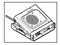
**6** Unplug the speaker cable from the socket on the main board to completely remove the top cover from the transceiver.
