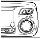
3 Rotate the DIAL to select [2 TX/RX], then press
