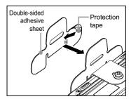
4 Install the bracket where you want to place the front panel.
