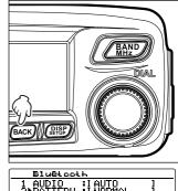
**8** Rotate the DIAL to select [2 BATTERY], then press DISP
