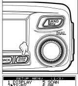
2 Rotate the DIAL to select [2 TX/RX], then press
