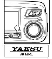
The entered call sign appears at the bottom of the screen, and the screen switches to the frequency display screen.
