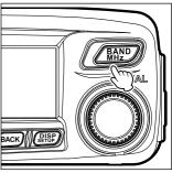
**3** Rotate the DIAL to select the desired memory channel.
