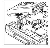
**7** Refer to the illustration on the right and carefully plug the FVS-2 into the connector.
