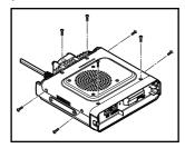
**5** Gently lift up the top cover of the transceiver from the rear edge.
