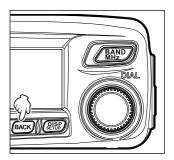
6 Rotate the DIAL to select [3 LCD CONTRAST], then press (DISP).
