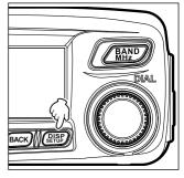
2 Rotate the DIAL to select [9 DATA], then press (SETUP).
