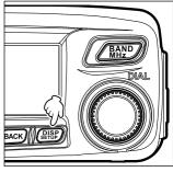
2 Rotate the DIAL to select [3 MEMORY], then press DISP SETUP.
