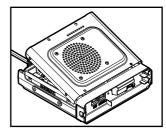
**6** Unplug the speaker cable from the socket on the main board to completely remove the top cover from the transceiver.
