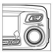
2 Rotate the DIAL to select [4 SIGNALING], then press DISP SETUP).
